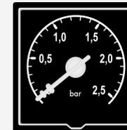
On the panel there is a gauge for the operating pressure in the collector. The pressure when the heat pump is not running should be between 0,5 and 2,5 bar. If the pressure falls below 0,5 bar a top up filling should be done.
